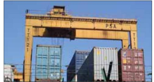
*A rail-mounted gantry crane of Tanjong Pagar terminal ready to lift a container*
